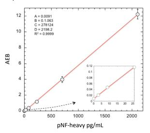
Lower Limit of Quantification (LLOQ): Triplicate measurements of serially diluted calibrator were read back on the calibration curve over 1 reagent lot on 1 instrument (5 runs total).
